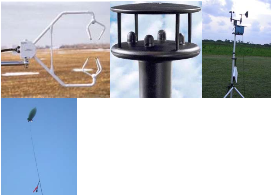
Fig 2 From left to right the is 1) the 3D sonic anemometer from Campbell Scientific 2) the 2D sonic from Gill, 3) the open field base station and 4) the kitoon at flight altitude. On the Kitoon tether flagged at the bottom of the picture is one of our ibuttons there top provide a temperature profile.
