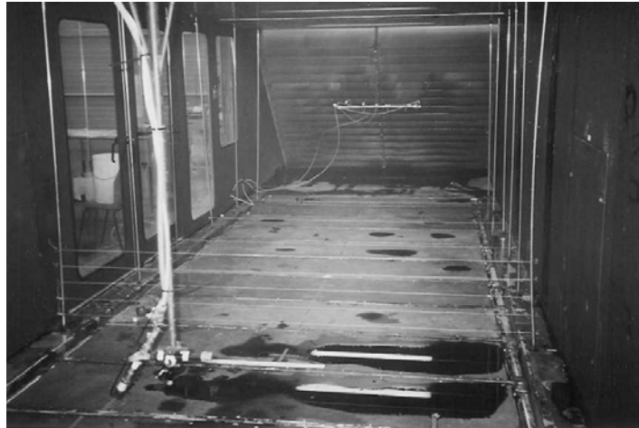
Figure 1. Inside view of SRI wind tunnel, vertical plane of DIX collectors, and horizontal plane of LERAP collectors
