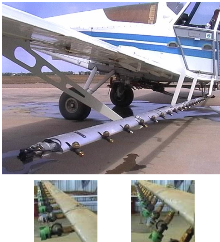
Figure 4. JARBA Boom showing the capacity of the nozzles to be rotated in flight (Jones Air)
