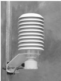
Figure 3. Shielded RH and Temperature Sensor R.M. Young Company (Courtesy John Campbell, R.M. Young Company, Traverse City, MI).
